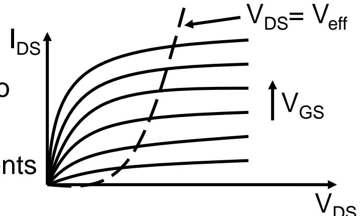
$$V_{\text{eff}2} = V_{\text{eff}3} = \sqrt{\frac{2I_{D2}}{\mu_n C_{\text{ox}} (W/L)}} = V_{\text{eff}} (\because I_{D2} = \frac{\mu_n C_{\text{ox}}}{2} \frac{W}{L} (V_{GS} - V_{\text{th}})^2)$$
