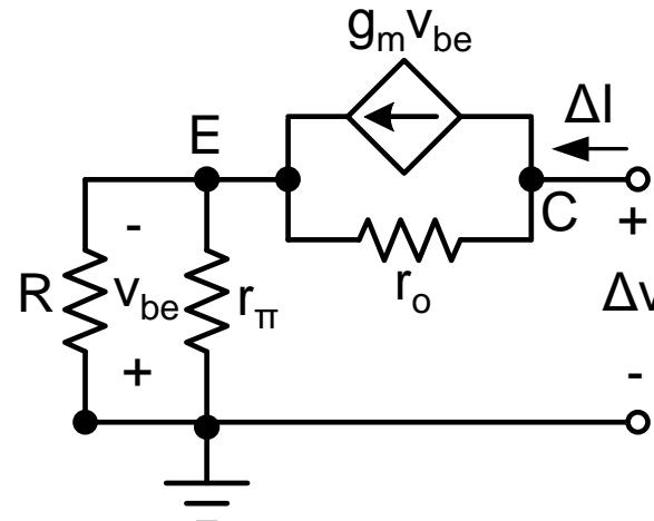
$$\Delta V = \Delta I(r_\pi // R) + [\Delta I + g_m \Delta I(r_\pi // R)]r_o$$
