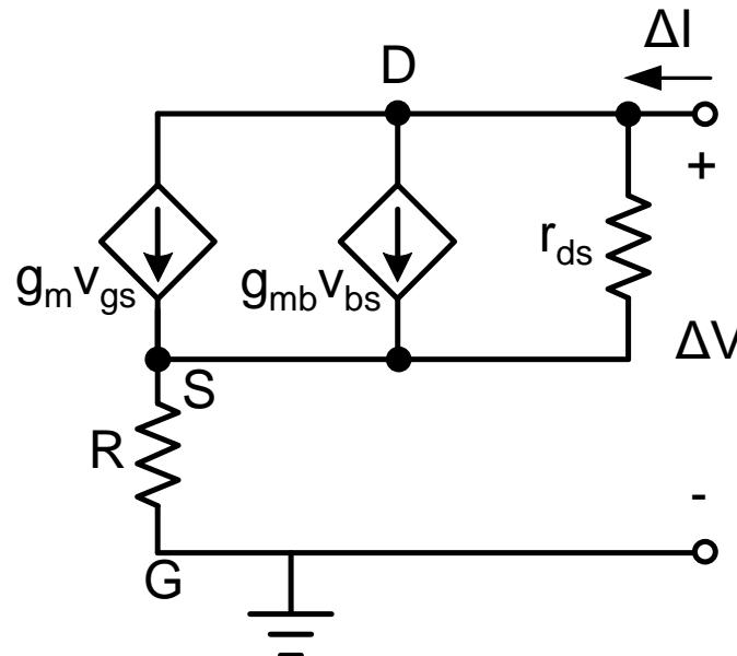
$$\text{Similarly, } R_o = \frac{\Delta V}{\Delta I} = r_{ds} [1 + (g_m + g_{mb} + g_{ds})R] \approx r_{ds} (1 + g_m R)$$
