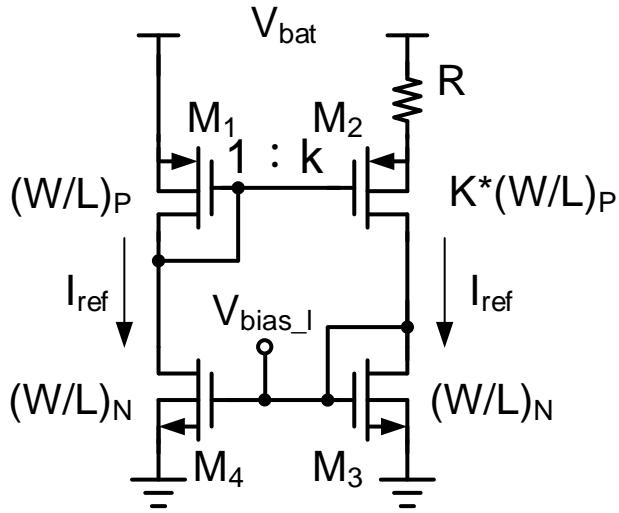
$$V_{SG1} = V_{SG2} + I_{ref} \times R$$
